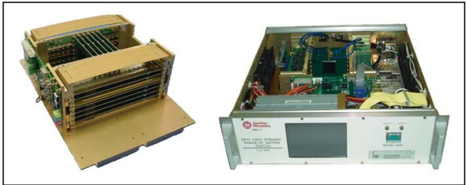
**Figure 2:** A solid-state (SS) RF matrix
